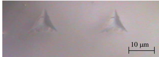
Figure 1 : Example of indent on resin surface.
