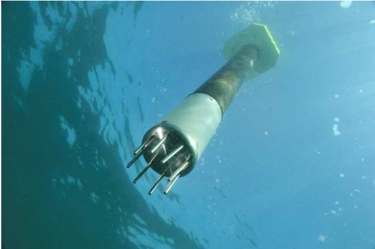
Arvor-C during the descent. On the bottom end, its claws prevent drifting when grounded on the seafloor
