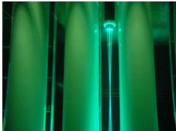
**Figure 2:** LDV measurement near the SMEC device of VerdErg Engineering Ltd
