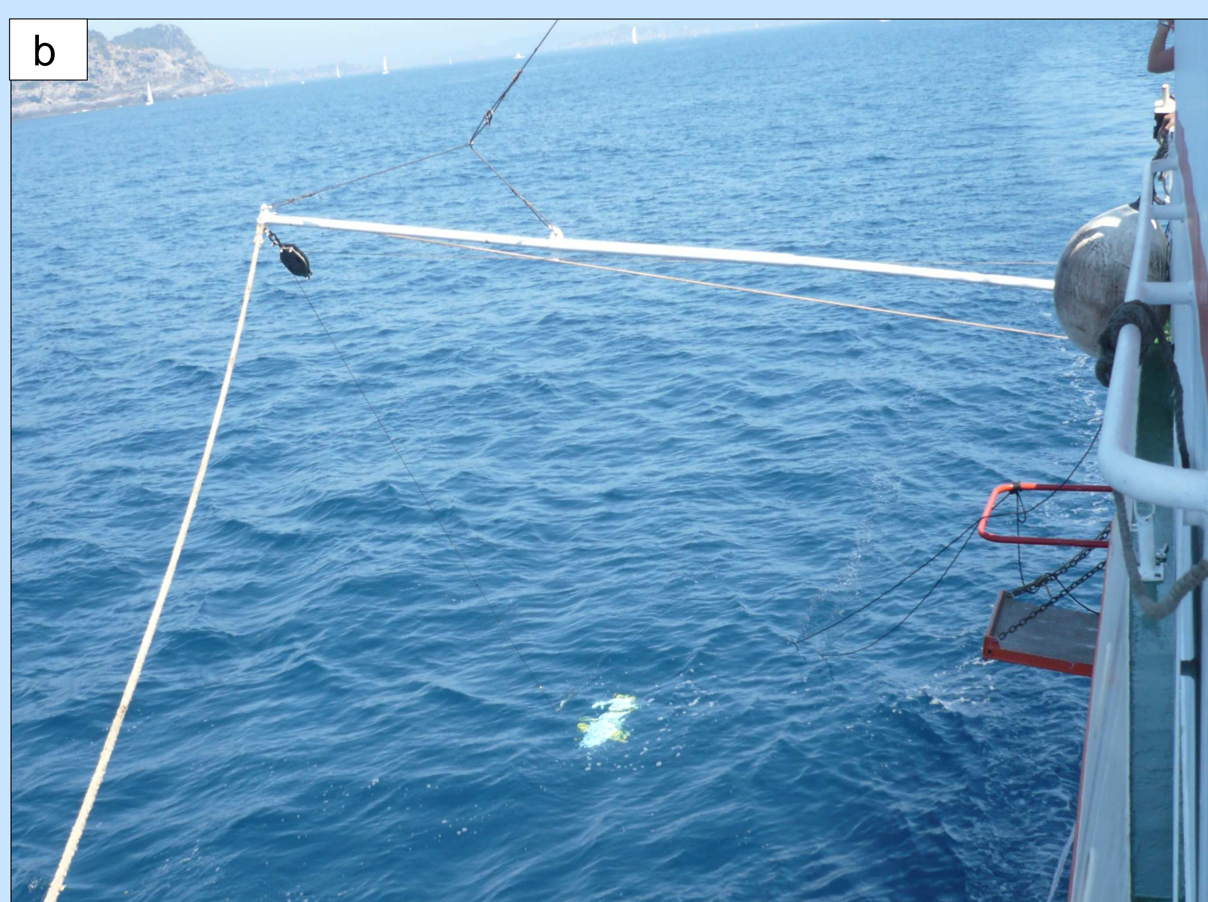
Figure 1 : a/ Launching of the towfish structure into water, b/ towfish structure installation on the starboard of the RV Téthys II.
