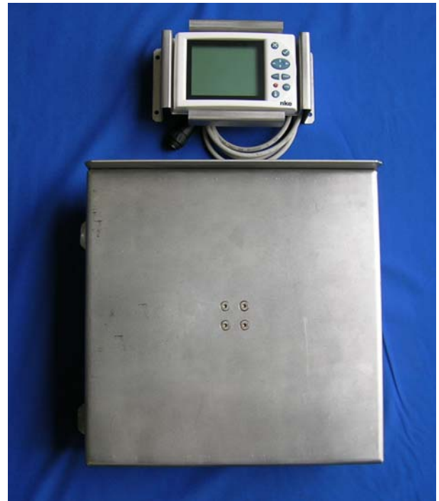
Picture 3: Recopesca weigh-scale (pan and command module)
