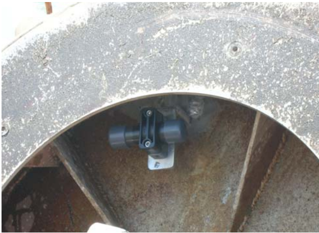
Picture 2: The "turns-counter" fixed in a gill-net hauler
