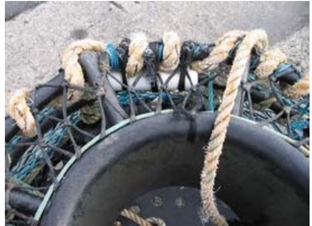
Picture 1b: Temperature-depth sensor fixed in a pot
