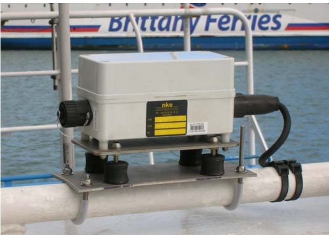
Picture 4: "Concentrator" of data onboard
