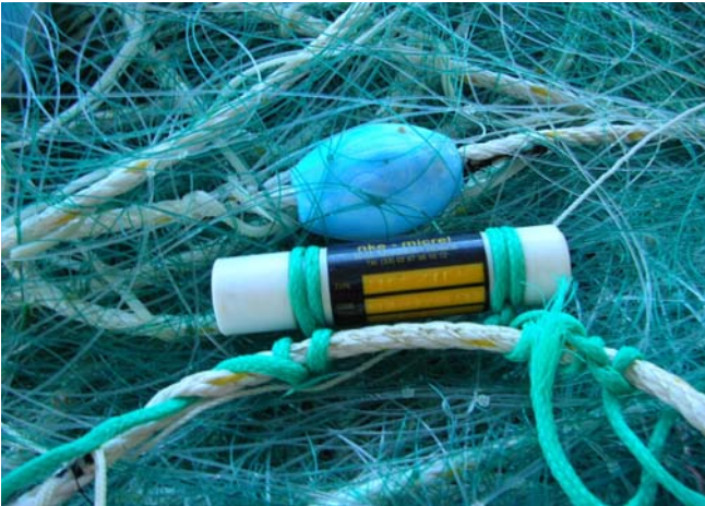
Picture 1a: Temperature-depth sensor fixed on a net
