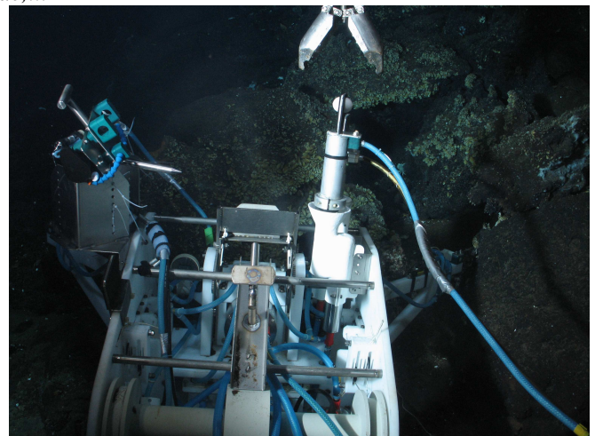
Seamon West was deployed at the base of the Tour Eiffel active edifice. The Tempo ecological module on the right is nearer. It includes a camera and lights, chemical analysers, oxygen optode,...
