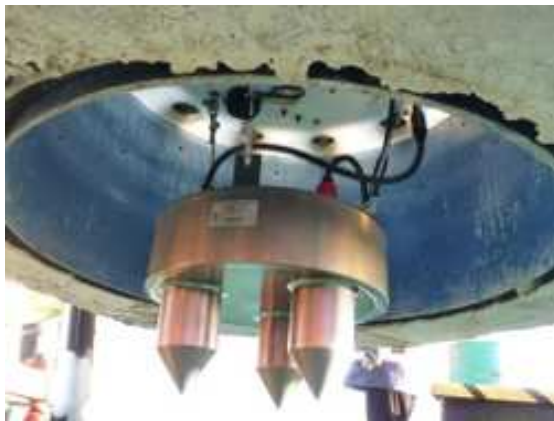
Concrete cap protecting the Guralp seismometer
