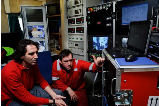
Figure 4-2. Left: The PEGASO ROV control system onboard the C/S Certamen (MECMA). Right: The PEGASO ROV de-attaching and cleaning ODI connectors installed at the NEMO-SN1 (Catania) cabled test site during sea operation.
