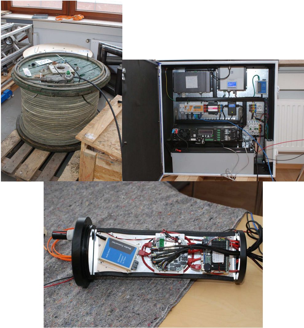
Figure 6.2: Top left – 600 m of ROV cable on a drum ready for deployment. Top right – view into the shore side cabinet containing the power supply and communication modules. Either UMTS or DSL lines can be employed to transmit data in real- time. Lower part – A view of the central underwater node with media converter for the fiber optic transmission and control electronics.
