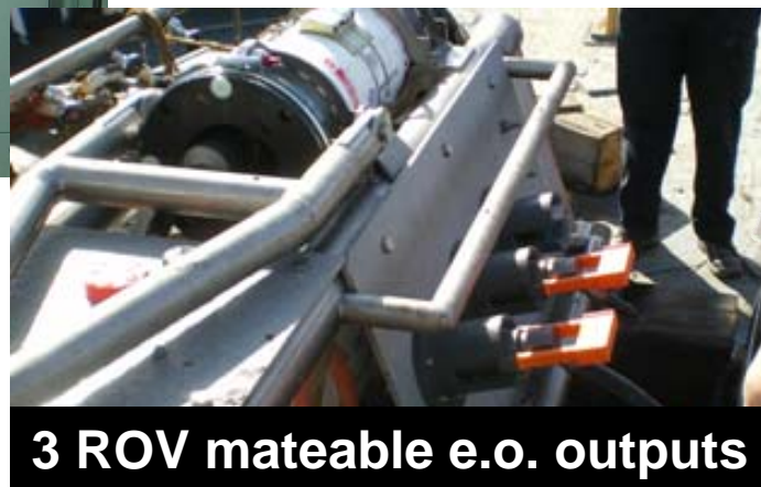
The Alcatel Junction Box 10 kVDC to 375VDC
