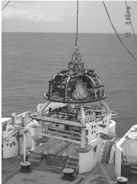
Fig. 3. SN-1 on board of C/V Pertinacia during the sea operations of deployment and connection to the cable (January 2005).
