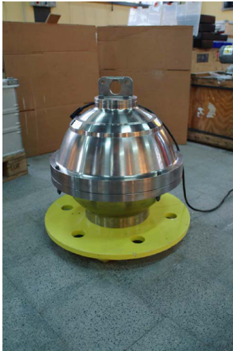
Fig. 6. The titanium-sphere containing the broadband seismometer.
