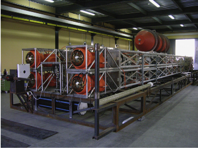
Fig. 3. The NEMO prototype tower fully assembled before its deployment.
