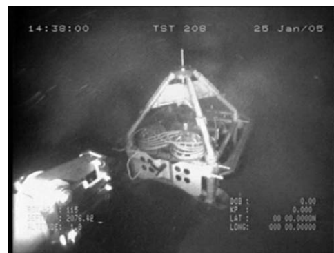
Fig. 5. ROV is approaching SN-1 for its connection to the electro-optical cable.
