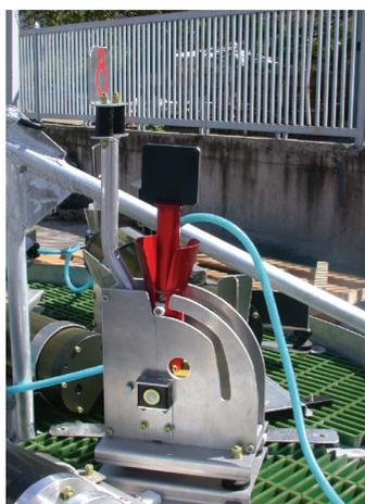
To ease the deployment, the OBS will be connected to SEAMON underwater using a low cost connection device (CdC,) specially developed and validated during the ASSEM project (Figure 5).
