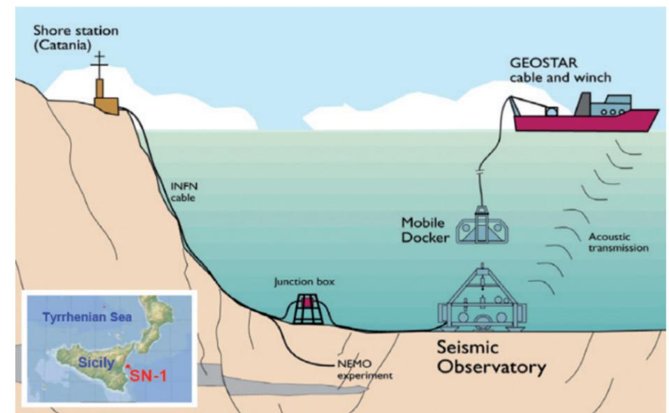
Figure 2 – Layout of the NEMO-SN1 underwater infrastructure in Sicily
