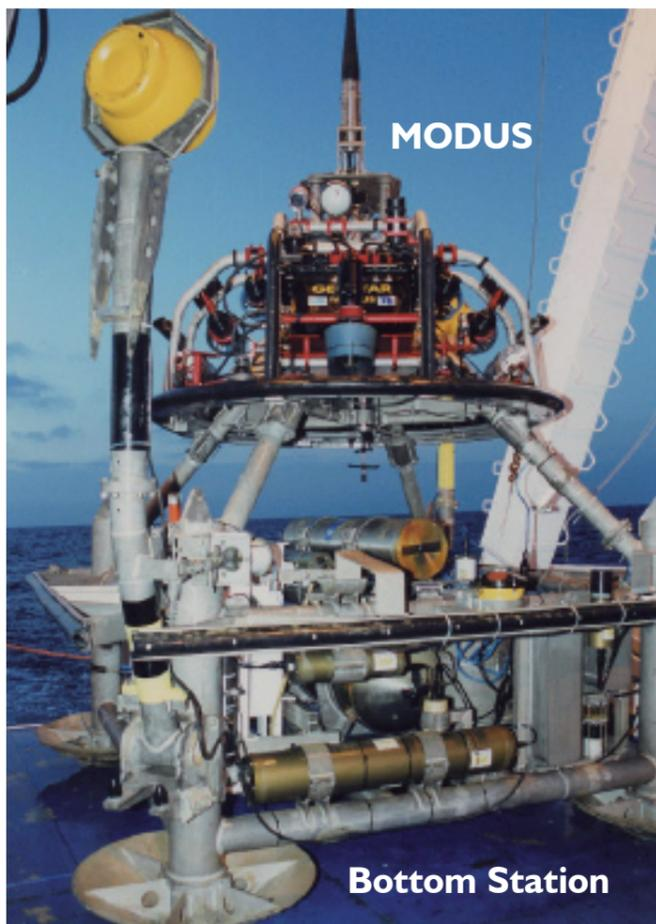
Figure 1 – GEOSTAR system: Bottom Station (bottom), MODUS (top)
