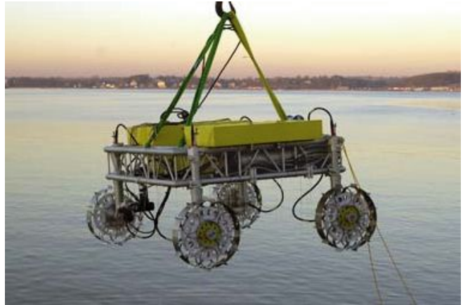
MOVE (Moving Lander) vehicle developed by DLR on behalf of the University of Bremen, shallow water test in the bay of Eckernförde
