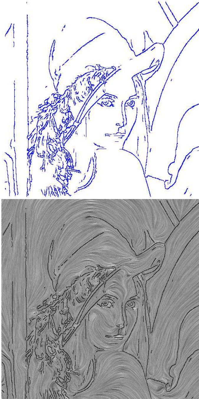
Figure 5: Test with the Lena image, initialised with the orthogonal to the gradient orientation field decimated using a Canny-Deriche filter. Notice that the recovered field is tangent to the edges, in particular at the top of the hat, on the strands of hair around the face and on Lena's jaw and chin.
