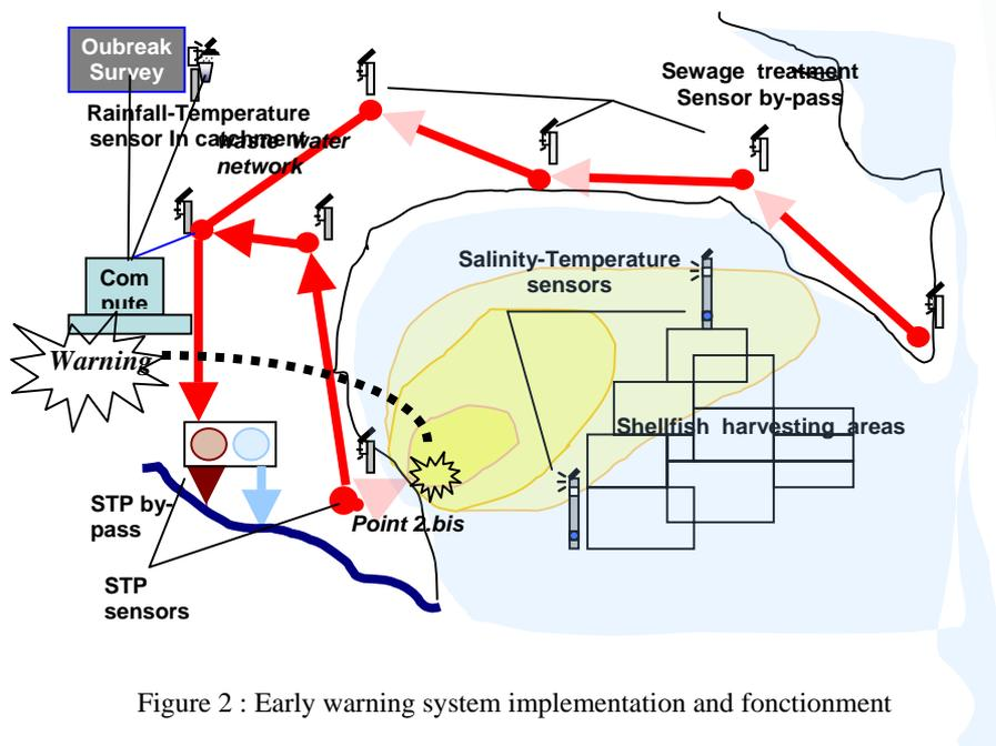
Figure 2 : Early warning system implementation and fonctionment
