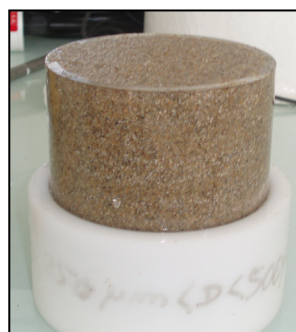
Sable grossier 300 \mu\text{m} < D < 750 \mu\text{m} D_{50} = 497 \mu\text{m} Teneur en eau = 0,26
