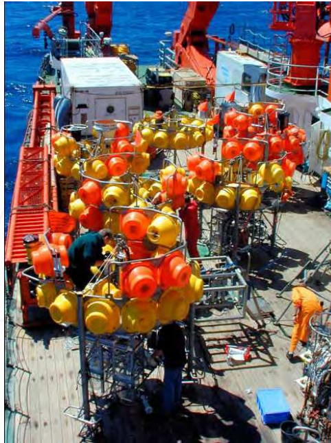
Fig. 2. Lander cluster developed by IFM-GEOMAR (source IFM- GEOMAR: http://www.ifm-geomar.de )
