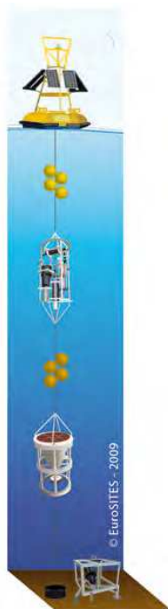
Fig. 11. A conceptual design of a EuroSITES open ocean observatory. (Source: EuroSITES)
