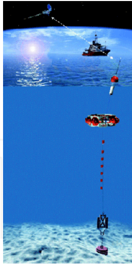
Fig. 6b. Concept of an Animate mooring (source: http://www.noc.soton.ac.uk/animate )
