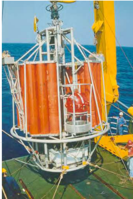
Fig. 3. NADIA observatory developed by Ifremer in 1985, © Ifremer
