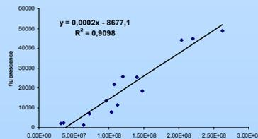
Fig. 6. Correlation between DAPI fluorescence measurement and DAPI stained bacteria counted by epifluorescence microscopy.
