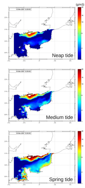
Figure 4: Evolution of SPM estimated by numerical model along a neap-spring tidal cycle in March 2007
