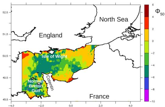
Figure2: Spatial repartition of median diameter  $\Phi_{50}$  in the computational domain ( $\Phi_{50}=\log(d_{50})/\log(2)$  with  $d_{50}$  in mm)
