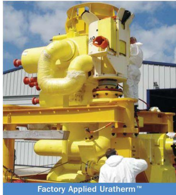
Figure 16 : Subsea structure insulated with GSPU material (courtesy Trelleborg)
