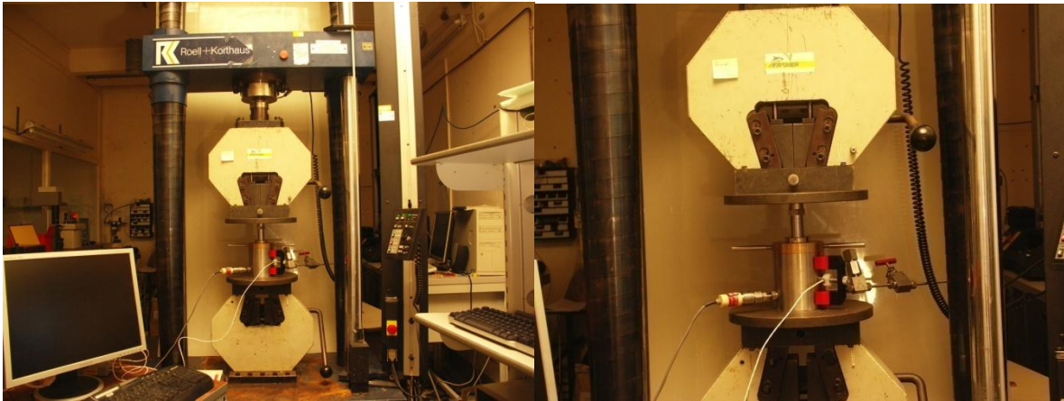
Figure 42 : Hydrostatic compression test based on piston displacement
