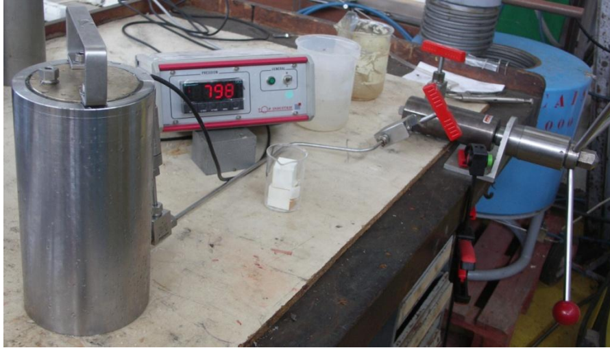
Figure 40 : Hydrostatic compression test based on volume change
