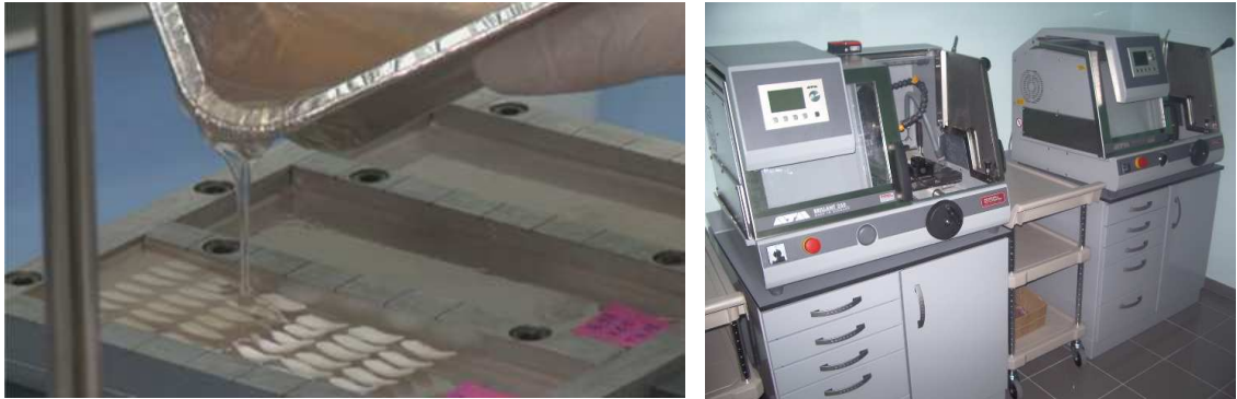
Figure 4: Inclusion of cod otoliths in resin and after they are cut by semi-automatic machine in Ifremer institute (France; In Mahé et al., 2009 ).
