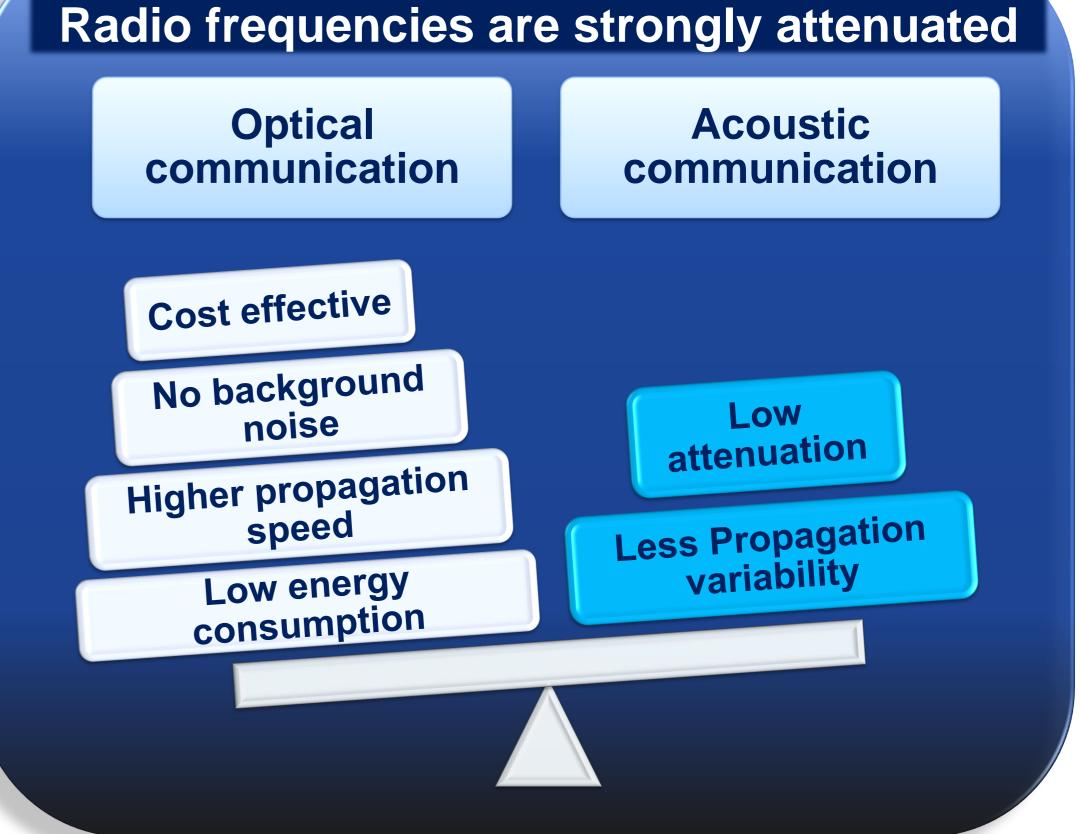
Absorption and scattering affect underwater optical signal propagation.
