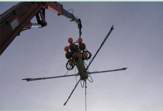
Fig. 1. The acoustic buoy with four hydrophones.
