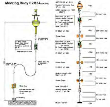
**Figure 2** – E2M3A configuration: surface buoy on the left (meteorological sensors + CT at 15m depth) and deep mooring scheme (CT, CTD and current-meters) on the right. The data presented in this work refer only to those collected by means of the deep mooring.
