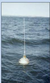
Fot. 1. A photograph of the Waverider buoy.
