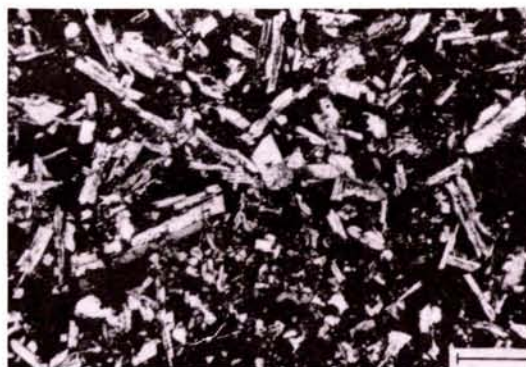
Figure 2a The weathered groundmass of Ceará rise sample 354-19-6 showing intergranular plagioclase, clinopyroxene, and oxides. Abundant layer-lattice silicate phases occupy the groundmass as weathering products. Crossed nicols; scale bar equals 1 mm.
