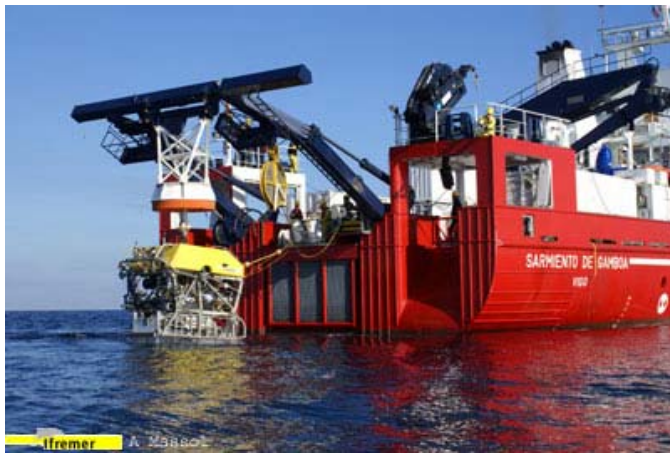
Figure 3. Mobilizing VICTOR 6000 on R/V Sarmiento De Gamboa (Photo: A. Massol, Ifremer).
