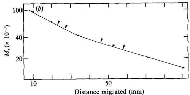
Fig. 5. (a) SDS-PAGE of RBV (Coomassie blue staining). Lane 1, RBV without Freon treatment; lane 2, RBV extracted with Freon; lane 3, protein markers. (b) Determination of the  $M_r$  of RBV polypeptides (arrows); protein markers (stars).
