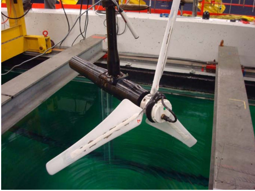
Figure 4: Turbine with 400mm blades and data logger before immersion, shown without nose cover
