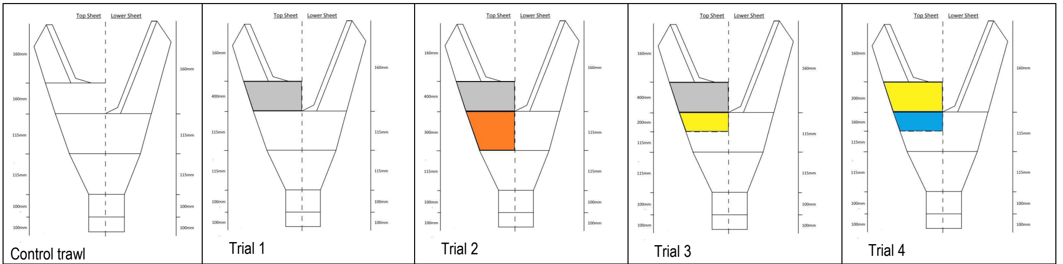
Figure 6.8.1. Net plans showing the different test configurations for the modified trawls. Large mesh panels inserted in the top sheet are highlighted in colours: grey (400 mm), orange (300 mm), yellow (200 mm) and blue (160 mm).
