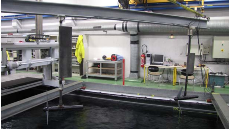
Figure 8: Photography of the experimental setup with a = 4D . For a > 5D configurations, the lengthwise girder is split into two smaller girders and two additional transverse girders are used to support them (cf. figure 9).
