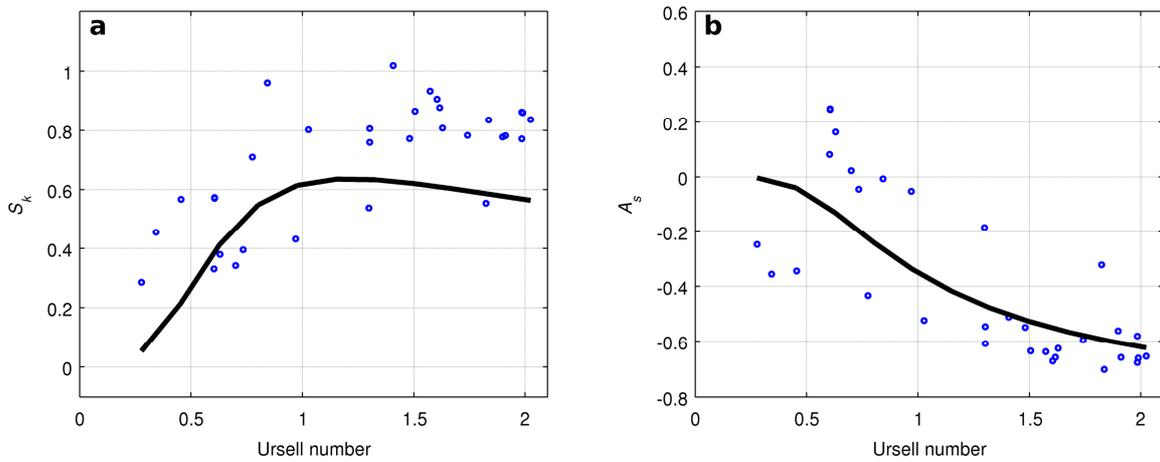
Figure 3. Velocity skewness ( $S_k$ ) and acceleration skewness ( $A_s$ ) versus Ursell number for the equilibrium barred-beach profile obtained in the LEGI flume. In both panels the model results and measurements are indicated by the solid black line and the blue circles, respectively.
