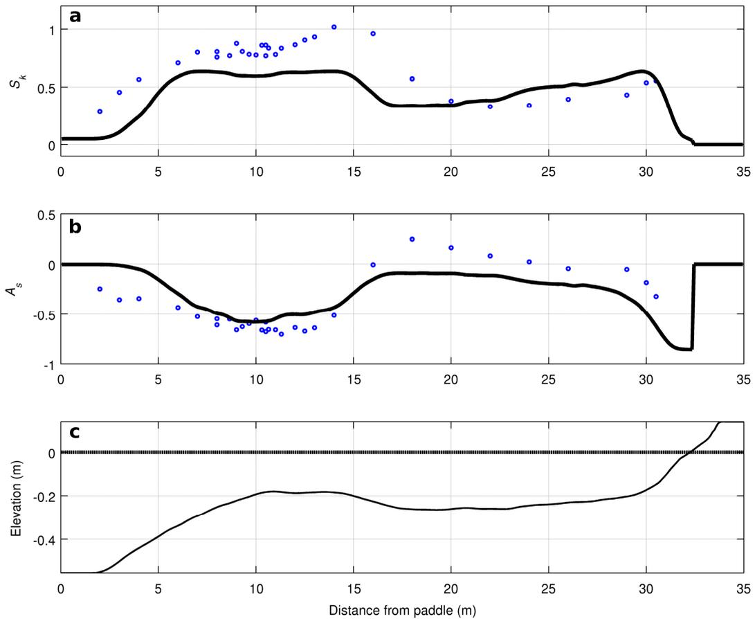
Figure 4. Cross-shore distribution of velocity skewness ( $S_k$ ) and acceleration skewness ( $A_s$ ) for the equilibrium barred-beach profile obtained in the LEGI flume. In (a,b) the model results and measurements are indicated by the solid black line and the blue circles, respectively.
