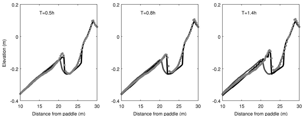
Figure 8. Simulation of the rapid onshore sandbar migration at  $t = 0.5, 0.8$  and  $1.4$  hours with best-fit free parameters determined through simulating annealing on this specific evolution. In all panels, model result (solid black line) and measurements (grey dots) are superimposed
