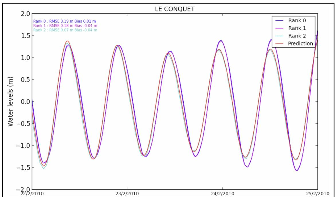
Figure 6: Comparison between modelled tide from rank 0, 1 and 2 models (without meteo) with predicted tide from observation at Le Conquet, from 22nd to 25th February 2010
