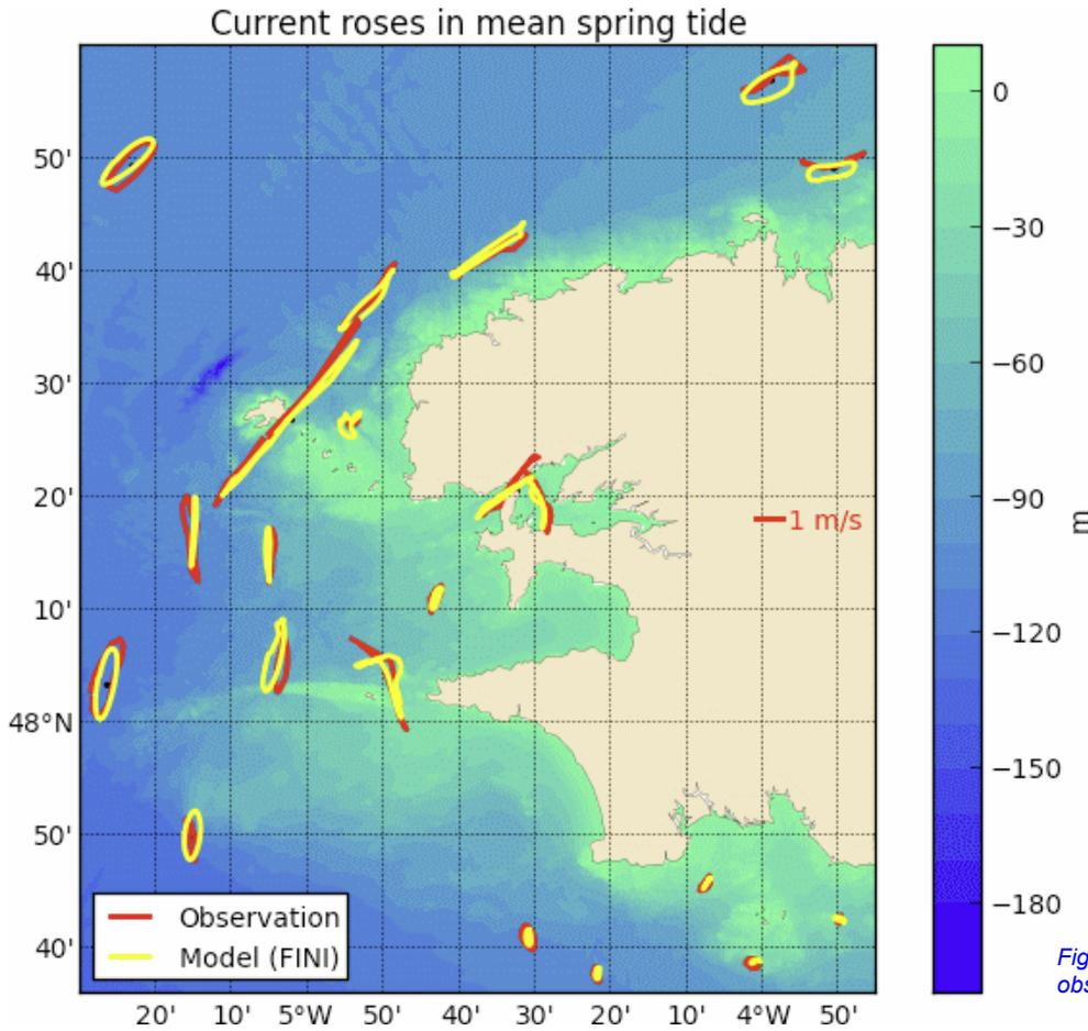
Figure 10: Comparison between modelled and observed current roses in mean spring tide
