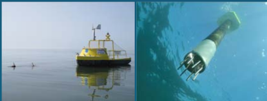
Large MAREL buoy (MOLIT) monitoring bottom and surface temperature, salinity, observed oxygen, fluorescence and turbidity. Coastal profiler measuring temperature and salinity (Arvor-C profiler).
