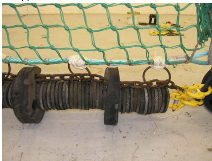
Figure 1. GOV lower wingend showing 5mm double PE guard netting and Ground gear D hoppers
