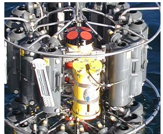
Upward-looking WH300 with the battery container on the side
