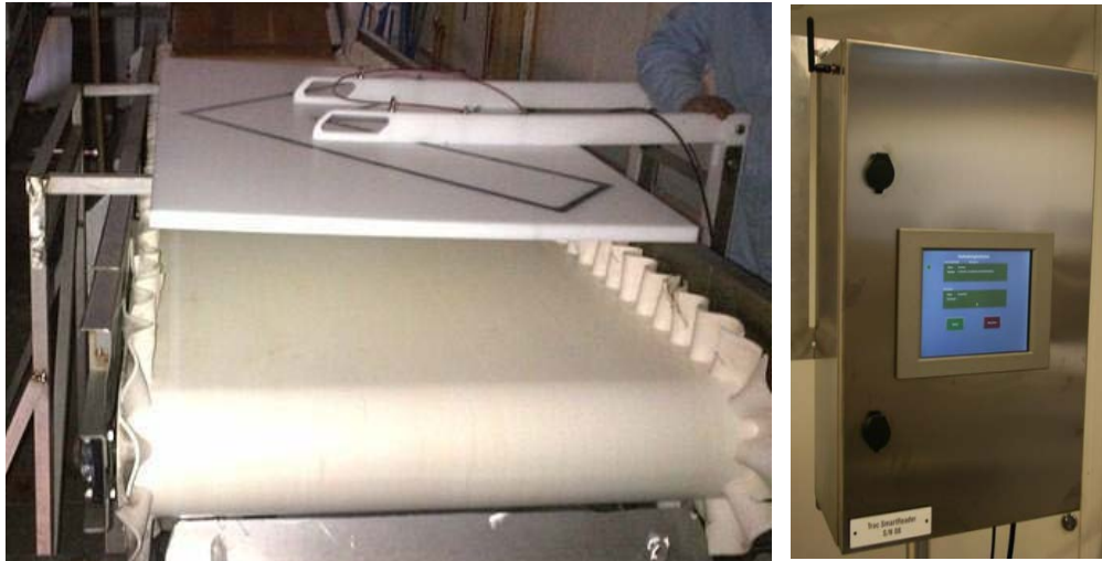
Figure 3.6.2.2.4. RFID antenna (left) and reader system with GPRS in a waterproof locker on the wall (right) that automatically detects RFID tagged fish and updates IMR database over GPRS with necessary data.
