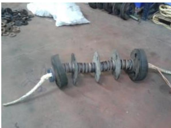
Figure 18: First version tested of light footrope.
