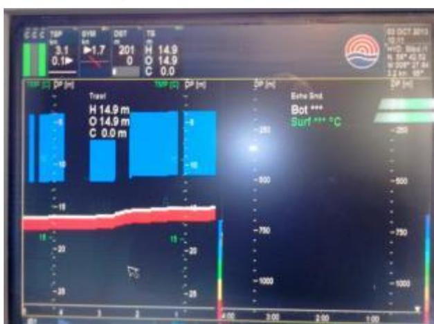
Figure 22: Scanmar screen showing the clearance value (“C 0.0” meaning clearance = 0 meter, also illustrated by the white line that would be off the red line in case of non nul clearance) during a trial with the light trawl adjusted to be towed off the bottom. On this diagram, the vertical trawl opening decreases of about 1 meter with no influence on the clearance.
