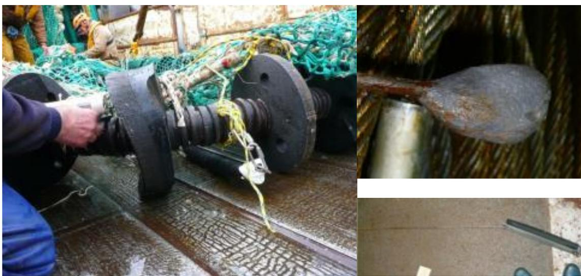
Figure 21: Dedicated sensor used to measure the distance between the footrope and the seabed. One of the steel bars was twisted once (for tow 21, bottom right picture). The lead mass appears to be used regularly which ensures its contact with the seabed (top right picture).
