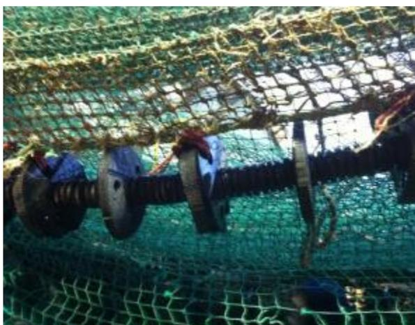
Figure 20: Connection between the rockhopper and the bolch line with ropes.
