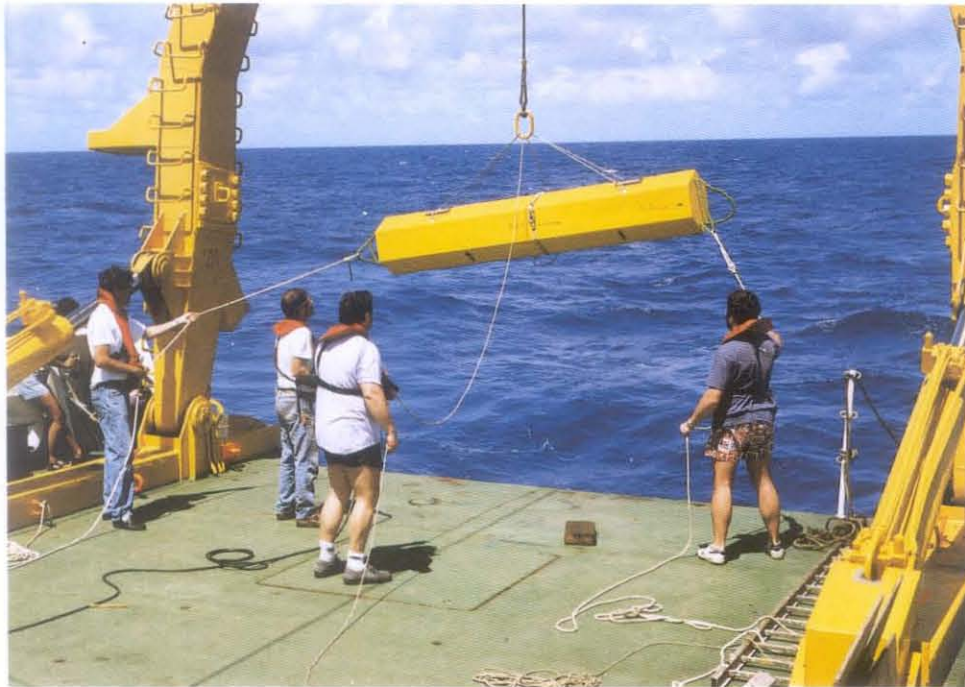
A MARVOR float is inside the yellow box. On touching the sea surface the box opens releasing the float (photo M. Ollitrault).
