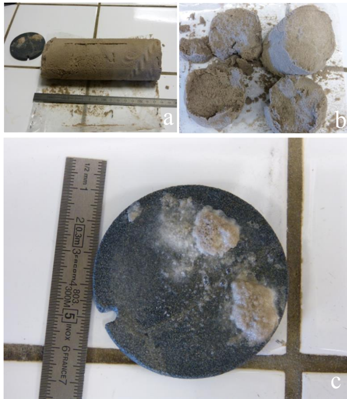
Figure 12. Methane-hydrate formation in a 5.82 % mass of clay-matrix and 94.18 % mass of sand.
