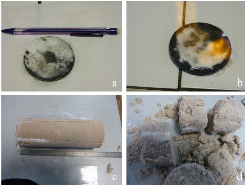
Figure 11. Methane-hydrate formation in silica sand: core retrieved from the vessel.
