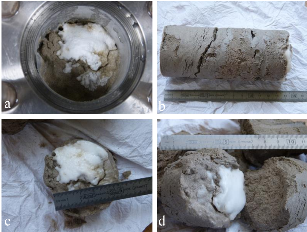
Figure 13. Methane-hydrate formation in a 19.80 % mass of clay-matrix and 80.20 % mass of sand.
