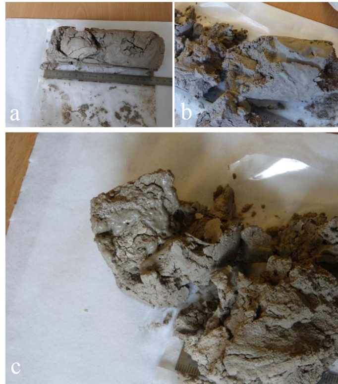
Figure 14. Methane-hydrate formation in a 40.35 % mass of clay-matrix and 59.65 % mass of sand.
