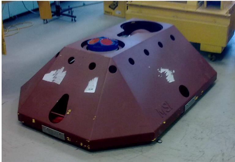
**Figure 2:** Example of an anti-trawl ADP bottom-mounting.
