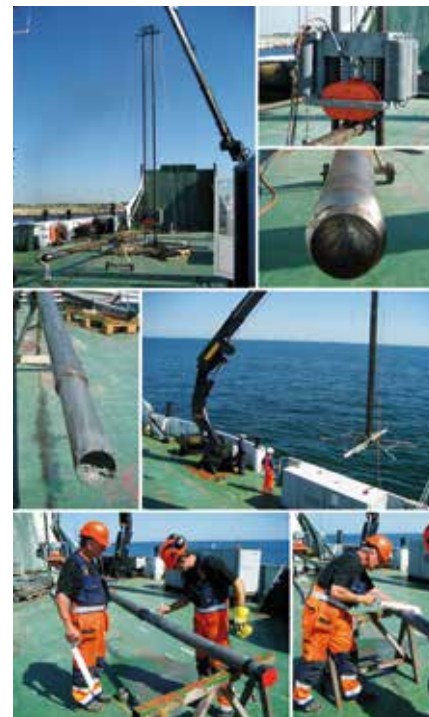
Fig. 4.10 Retrieval of sediment cores in the Fehmarnbelt-project for geological and palaeoenvironmental investigations.
