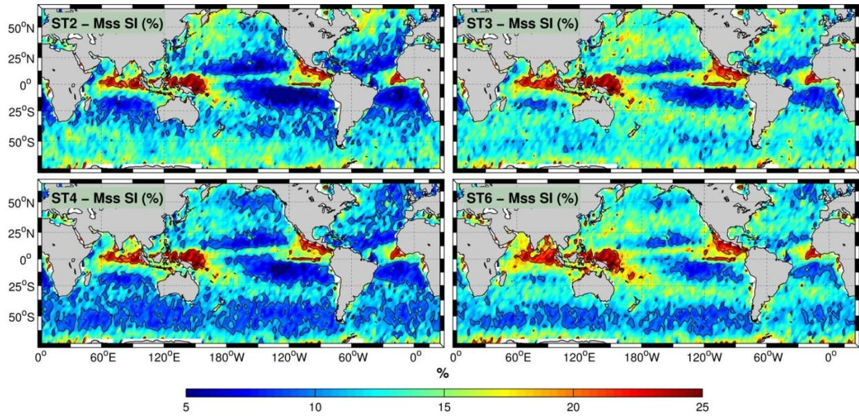
**Figure 4:** Scatter indices (in percentage) for ST2, ST3, ST4, and ST6 using co-located mean squared slopes from ENVISAT for 2011 gridded in 2° bins.
