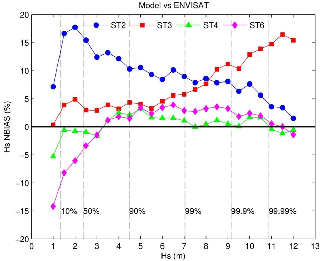
**Figure 5:** Normalized wave height bias (in percentage) for ST2, ST3, ST4, and ST6 plotted in terms of sea state ( $H_s$ ).
