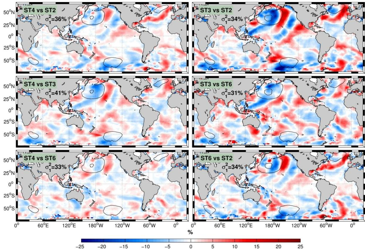
**Figure 11:** Spatial distribution of the first Eigen vector of the empirical orthogonal functions (EOFs) between source terms ST2, ST3, ST4, ST6. EOFs were computed from a time series from 17-20 January 2011. Solid contours indicate large sea states (5 and 10 m wave height).
