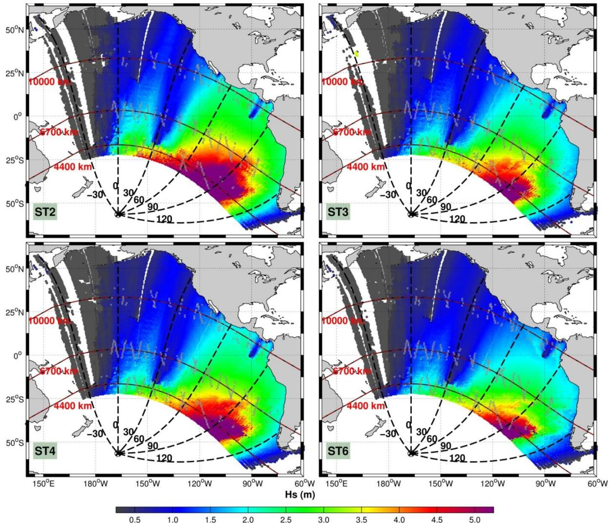
**Figure 12:** Spatial distribution of the swell wave heights (in meters) from the generation source (167°W, 56.5°S) on August 24, 2011 1200UTC for ST2, ST3, ST4, ST6. The dashed black lines represent great circle routes with the same wave heading from the source. The dashed red lines represent equidistant from the source. The stipulated grey points represent co-located ENVISAT SAR wave partitions.
