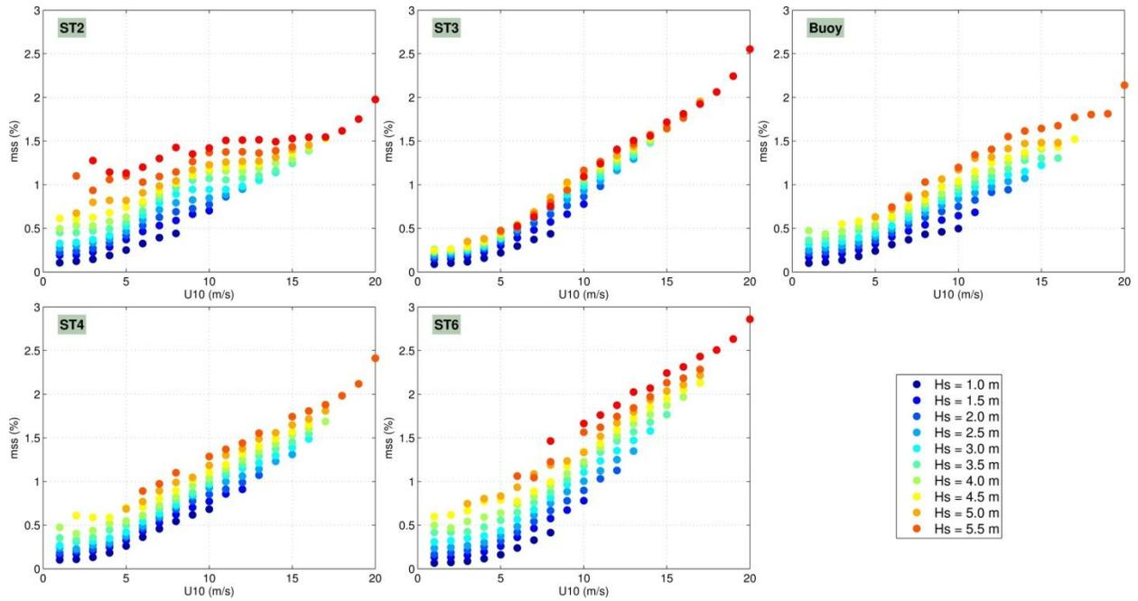
**Figure 7:** Variation of the surface mean square slope estimated from all buoys from 0.037 to 0.485 Hz. Wind speeds at 10 m height are estimated from the buoy using a logarithmic wind profile and averaged into 0.5 m/s bins while wave heights are averaged into 0.5 m bins to estimate the average mean square slope.
