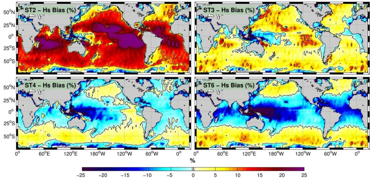
**Figure 3:** Normalized wave height bias (in percentage) for ST2, ST3, ST4, and ST6 using co-located wave heights from ENVISAT for 2011 gridded in 2° bins.
