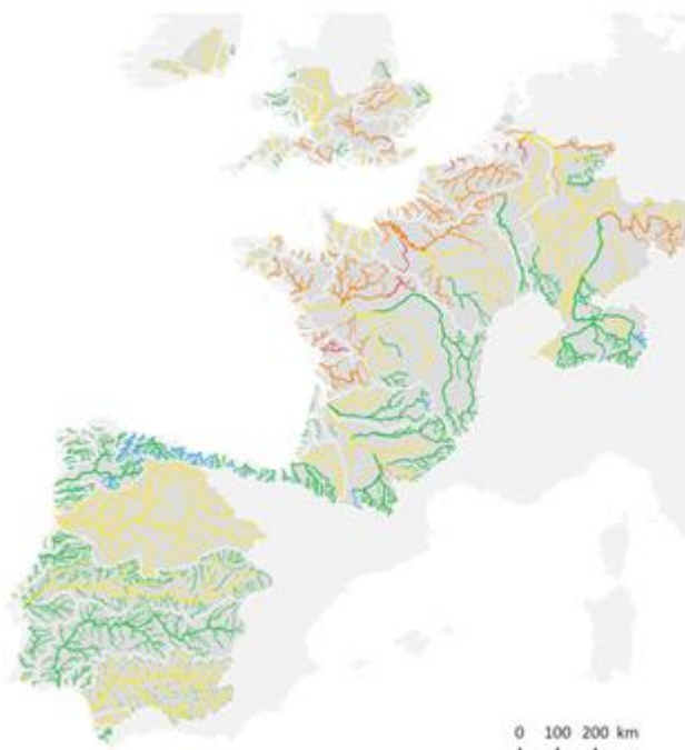
Figure 47: Annual mean concentrations of NO 3 in the NEA domain simulated for the Reference scenario.
