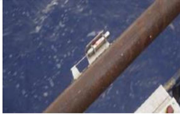
**Figure 28: VHP probes in its support welded to the pipe of the coring system.**
