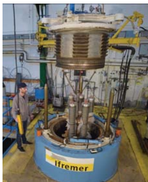
Figure 1 : Qualification en pression des tubes (composites) Deep-Arvor.
