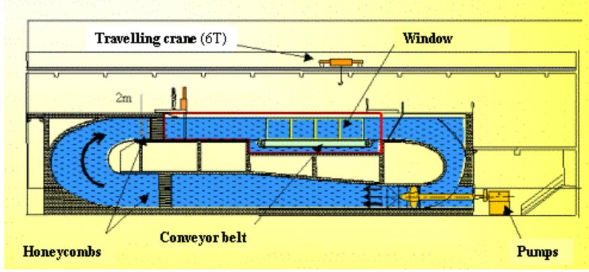
Figure 1: Schematic view of the wave and current circulating tank
