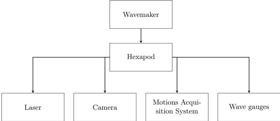
Figure 9: Synchronism diagram of the experimental set-up between the wavemaker, the hexapod and the dedicated instrumentation
