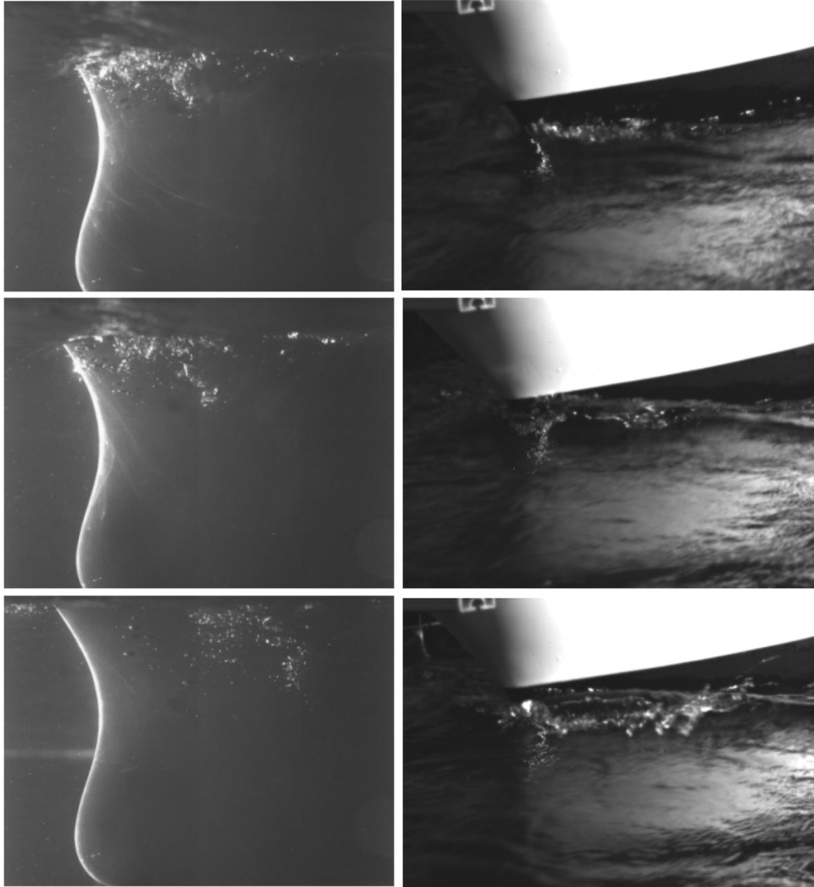
Figure 13: Simultaneous visualizations of the generation of bubbles (left) and the breaking wave (right) during the breaking wave event ( $t_1$ ,  $t_2$  and  $t_3$ ).
