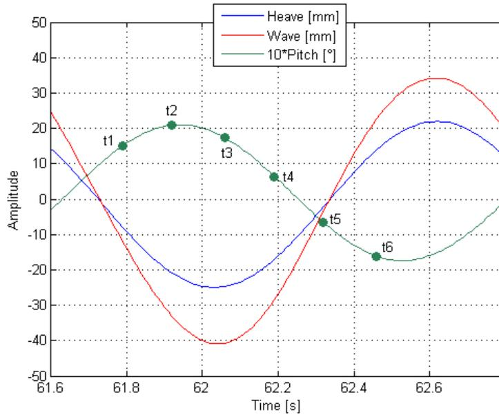
Figure 15: Pitch, heave and free surface elevation (at the center of gravity) during instantaneous visualizations ( $t_1 \rightarrow t_6$ ) of breaking wave and air entrainment events.
