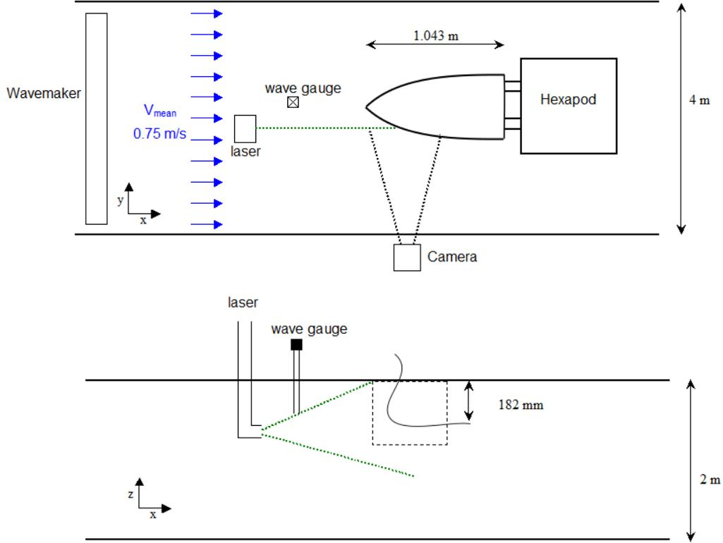
Figure 6: Drawing of the experimental set-up, top and side view showing the light sheet generation system location
