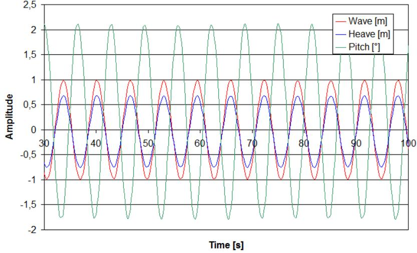
Figure 8: FREDYN results for the trial conditions at real scale
