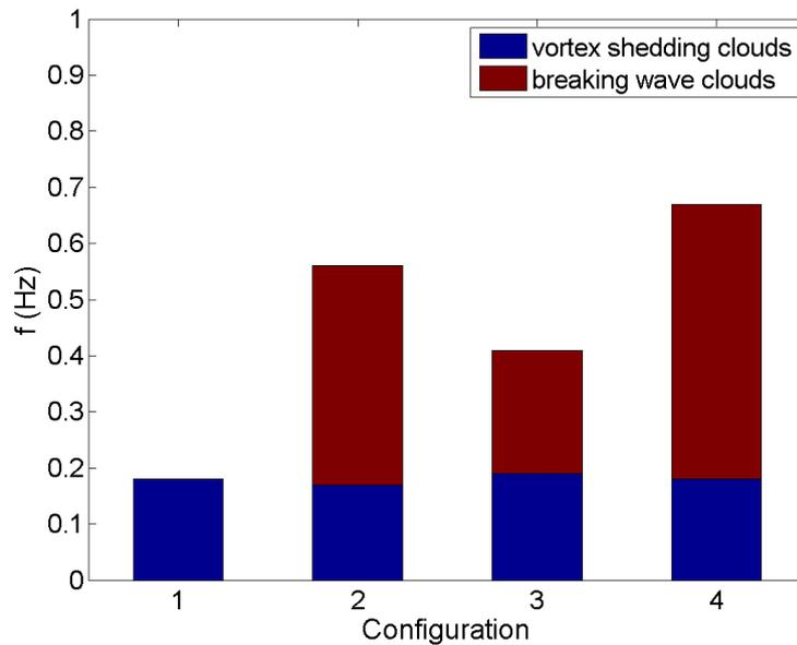
Figure 16: Air entrainment frequency, breaking wave clouds and vortex shedding clouds, for the 4 test configurations
