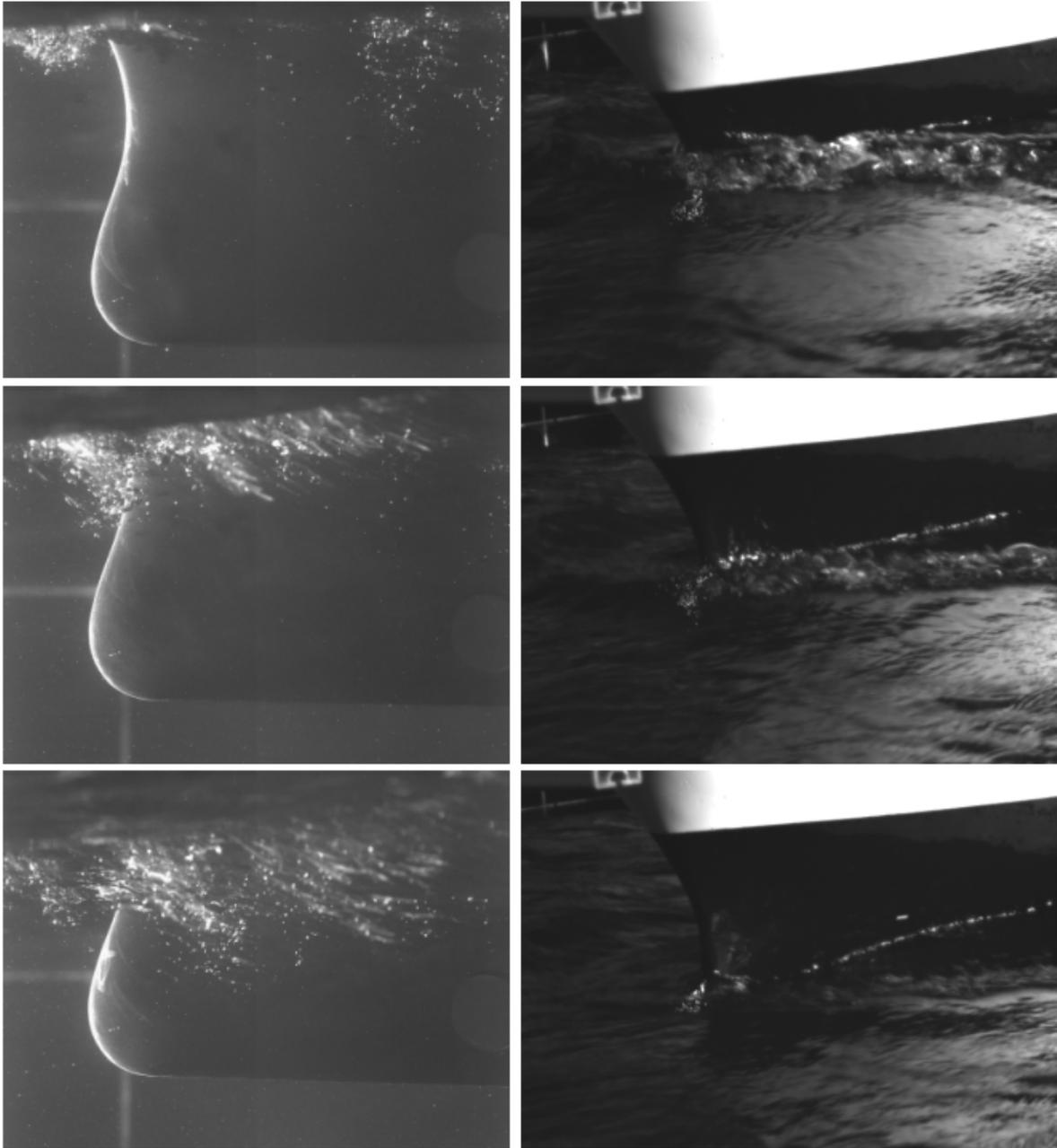
Figure 14: Simultaneous visualizations of the generation of bubbles (left) and the breaking wave (right) during the breaking wave event ( $t_4$ ,  $t_5$  and  $t_6$ ).
