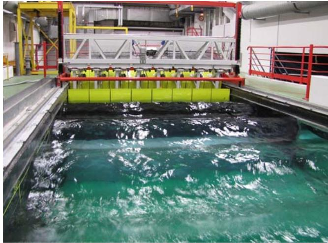
Figure 7: Illustration of regular wave generation in the tank with a current of  $0.75 \text{ m/s}$
