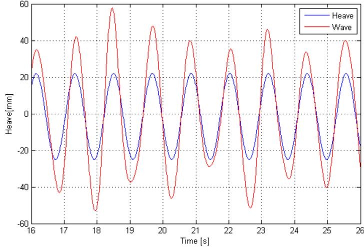
Figure 10: Example of waves and heave synchronisation from the experimental measurements with a current of 0.75 m/s
