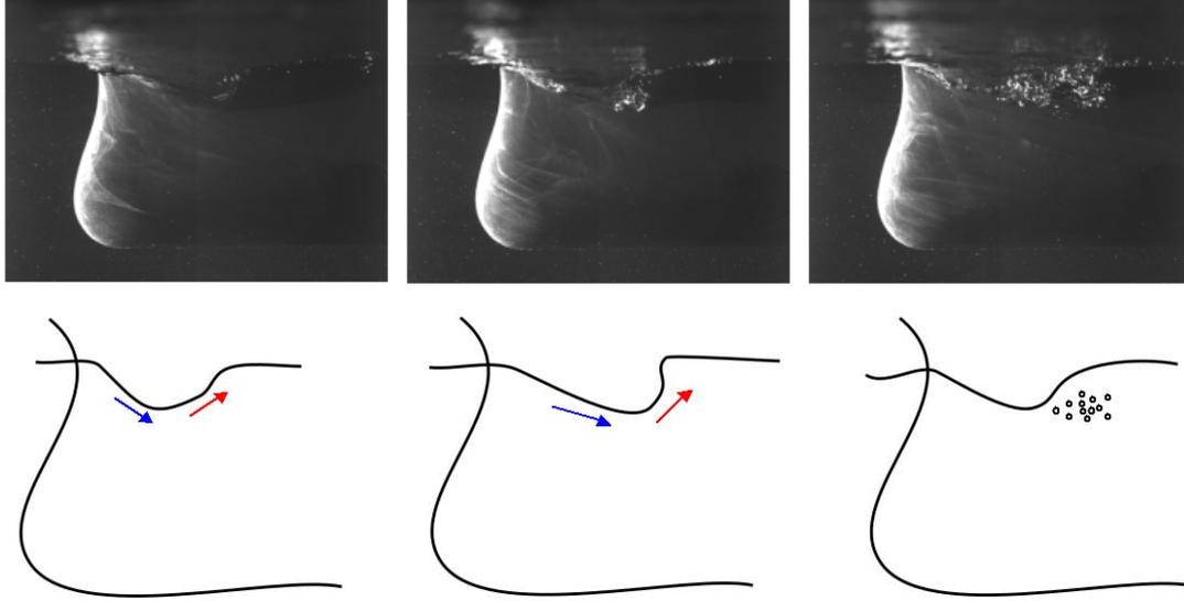
Figure 11: Description of the vortex shedding clouds generation from the free surface distortion to the flow aeration, encountered in the fourth cases
