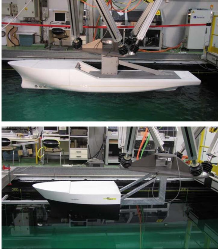
Figure 2: 1/30 model of the *Pourquoi pas?* fixed under the hexapod. Top: full model. Bottom: bow model only with the same relative position to the hexapod center of reference than for the full model
