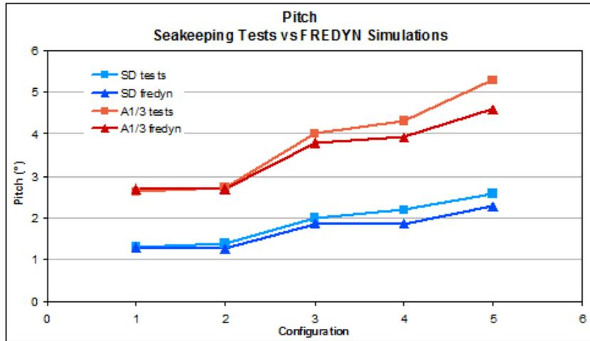
Figure 4: Comparison of Fredyn and seakeeping test results for several sea state conditions
