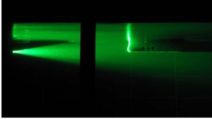
Figure 5: Laser sheet in the ship model axis for the acquisition system in the bow vicinity of the *Pourquoi pas?*
