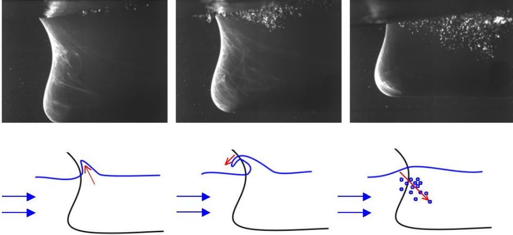
Figure 12: Description of the breaking wave clouds generation from the generation of a reflective wave on the bow to the flow aeration, encountered only for case 2 to 4
