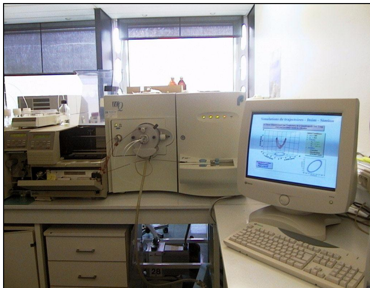
Figure 3 : Ensemble de couplage CLHP/SM) n , ThermoFinnigan (F. Mondeguer, DEL/PN, Ifremer, Nantes).
