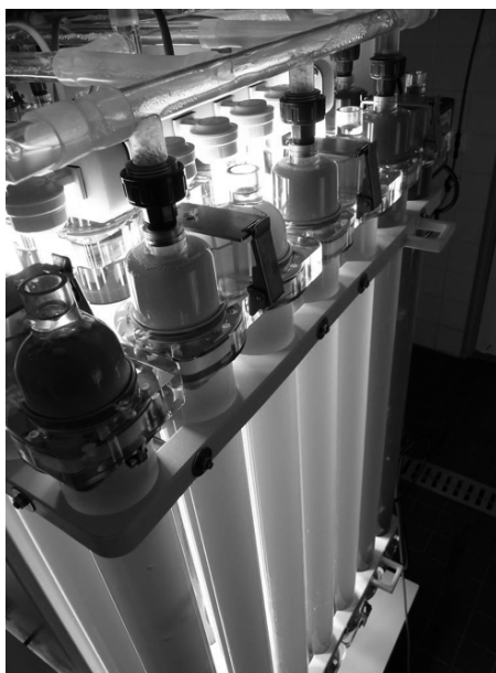
Figure 2.7. Photobioreactor JSP-120 for the automated production of microalgae in marine mollusk hatcheries (photo Kaas/Ifremer)
