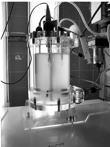
Figure 2.8. Photobioreactor with instrumented turbine, used in ecophysiological studies in controlled conditions (photo Kaas/Ifremer)
