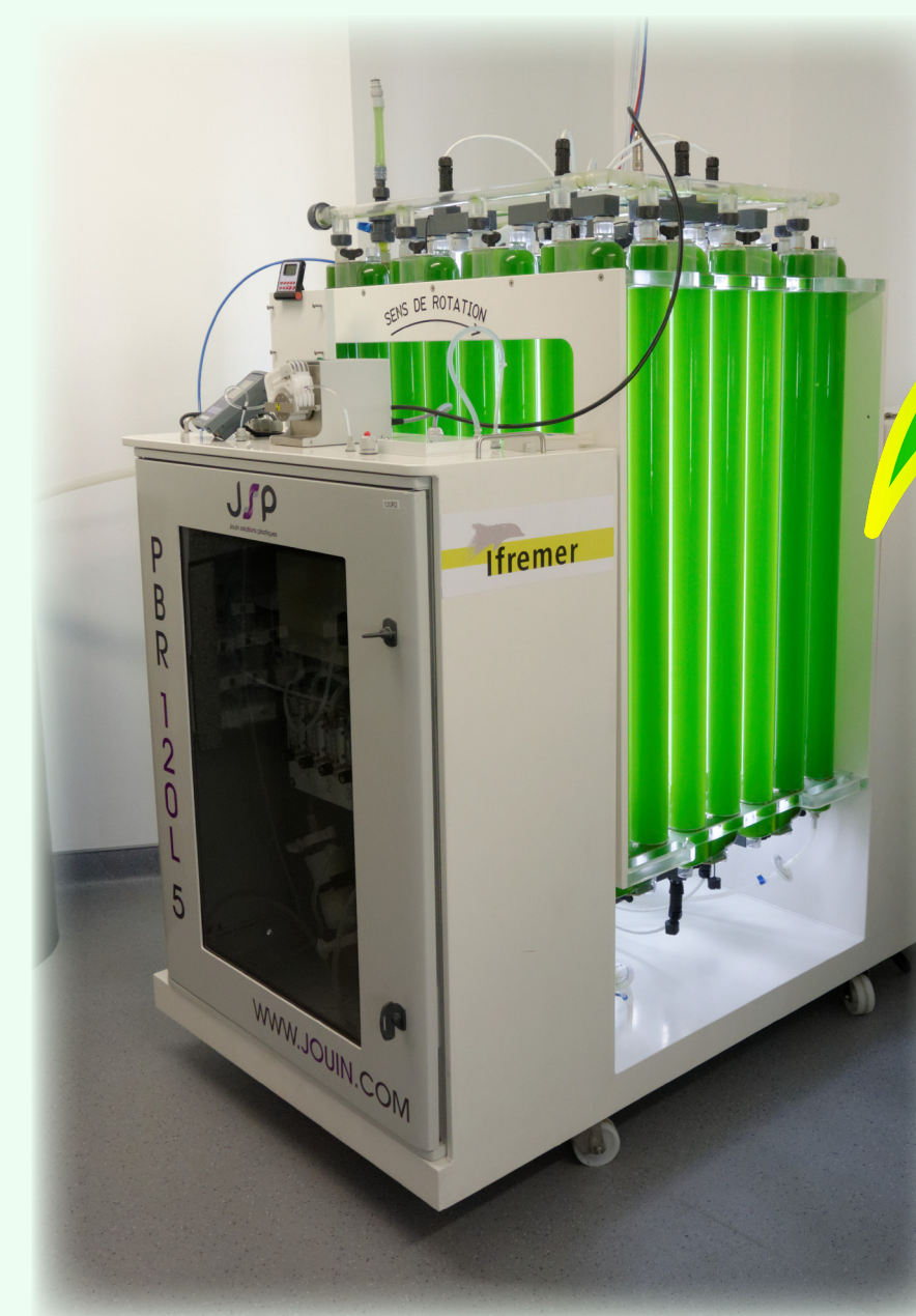
Figure 1 : culture of microalgae in a photobioreactor.
