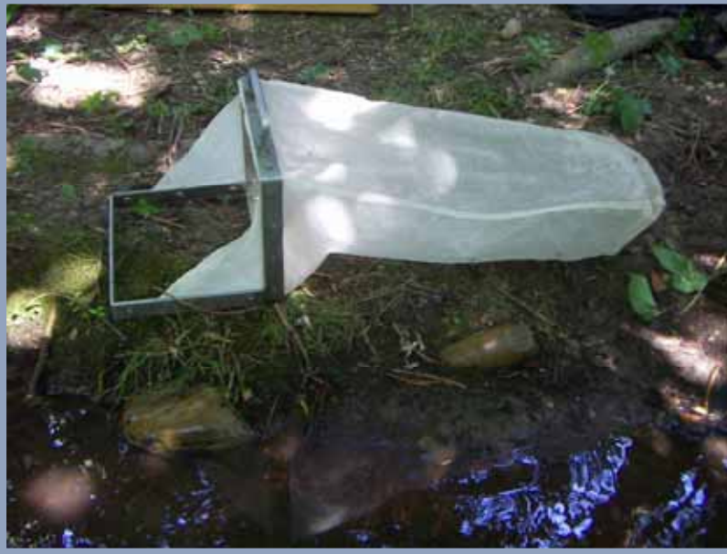
Figure 1: IBGN Surber sampler
