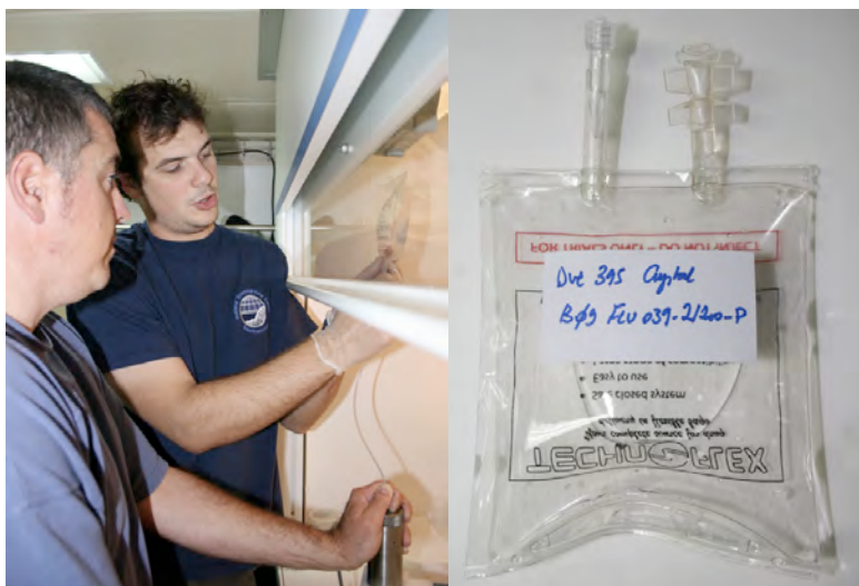
Figure 3: Example of gas collection from gas-tight Ti-bottles (left inside) and of gas pocket (on the right inside).
