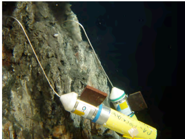
Figure 2 : A picture of two high-T probes with their yellow handle and their wood plate in vents.
