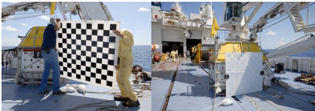
Figure 7 - Attachment of the OTUS calibration grid to the NASA.
