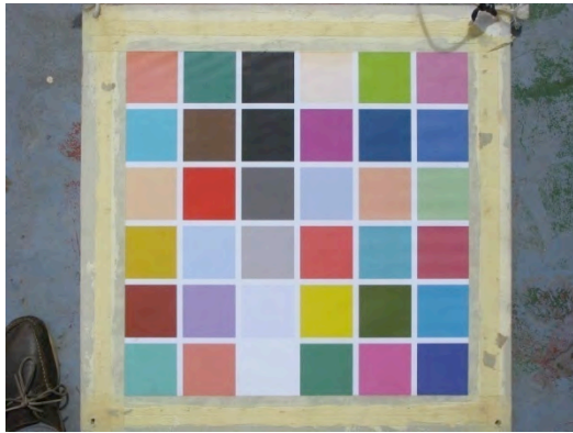
Figure 15 - Image of the color chart at the surface that was used as a reference for the corrected color values.
