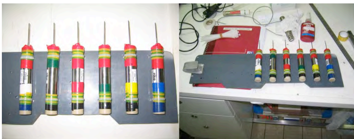
Figure 4 : Array of 6 low-T probes mounted on a Plexiglas plate to measure temperature gradients in hydrothermal plumes.
