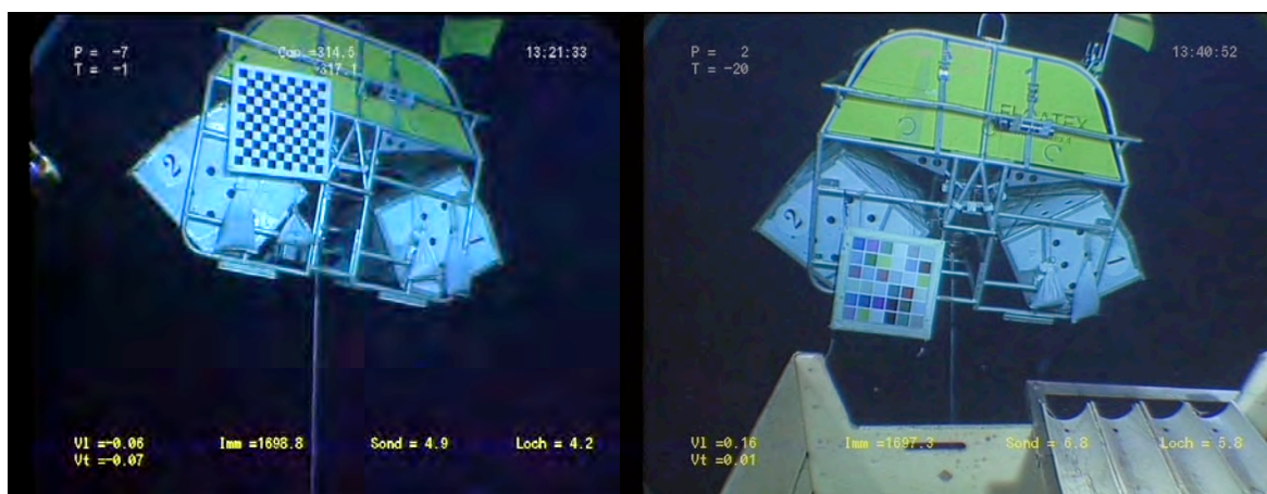
Figure 13 - Double sided calibration grid attached to the NASA, arranged for geometric calibration (left) and color calibration (right).
