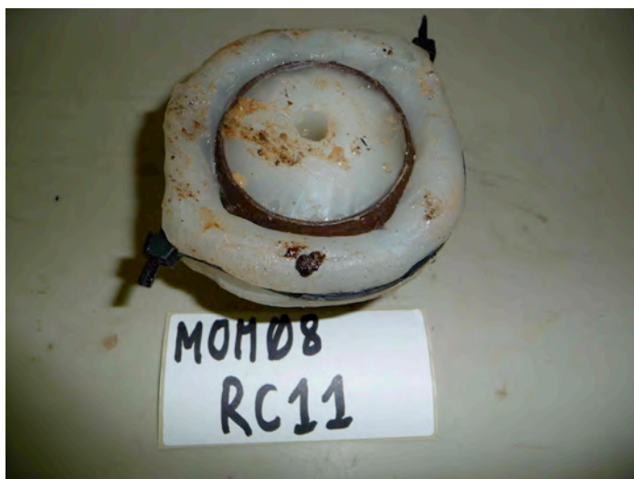
Figure 1: sediment-core head prepared for rock-core. The diameter of the head (without the ring of wax) is ~8 cm. The ring of wax is fixed with tie-wraps. The wax is surf wax from the company “sticky bumps” (USA).
