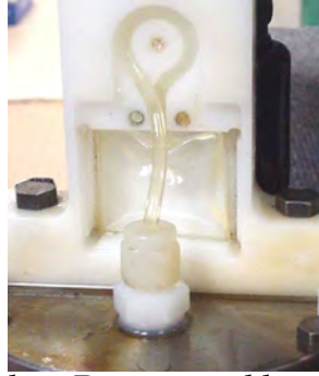
Canule + Pressure oil bag Photo SBE53 (manual page56)
